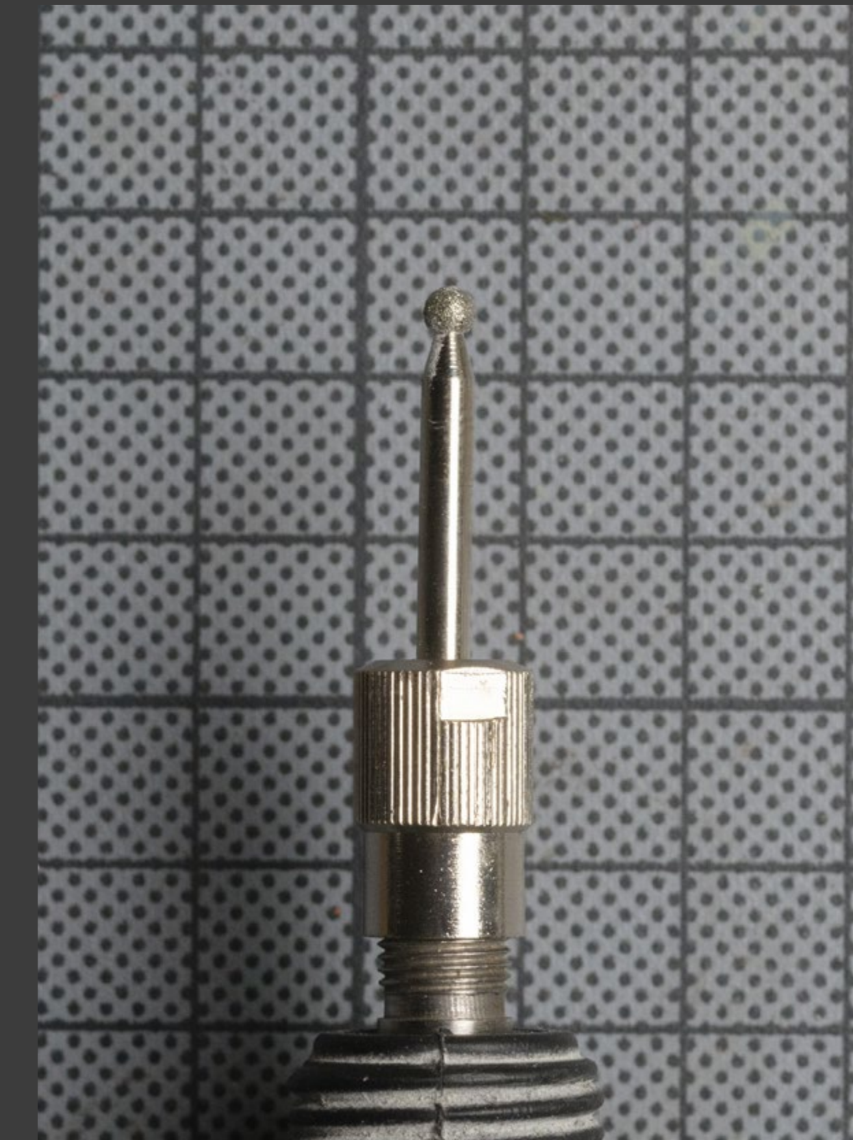
3mm ball gouge for a dremel. You could also use a hand drill and work the edges with a hobby knife.
