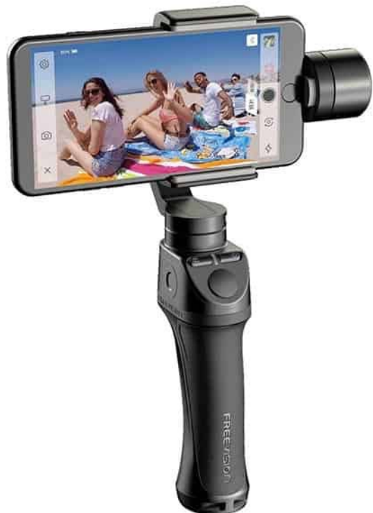
A GIMBAL STEADIES A CAMERAPHONE USING THREE BLDC MOTORS, ONE ON EACH AXIS.
